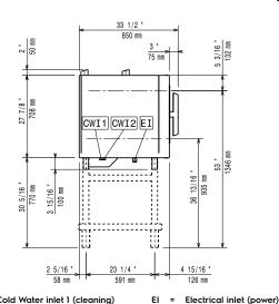
Cold Water inlet 1 (cleaning) CWII CWI2 Cold Water Inlet 2 (steam
